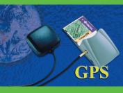
Pretec CompactGPS<sup>™</sup> is the world's smallest GPS card in CompactFlash package. With the mapping system bundled with your PPC, HPC, or notebook computer, it can track all satellites in views and provide accurate positioning wide range of applications including transportation, marine, aviation, and industrial
